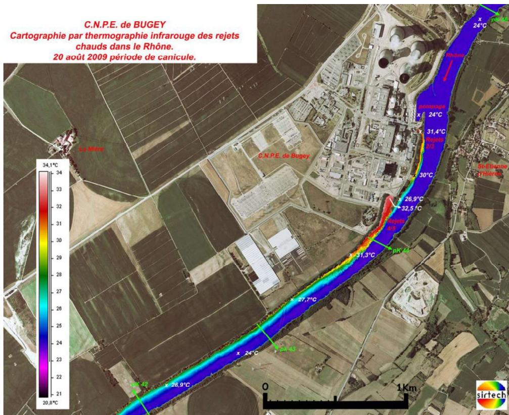
**CARTOGRAPHIE THERMIQUE DES REJETS CHAUDS DU CNPE DE BUGEY DANS LE RHÔNE**
